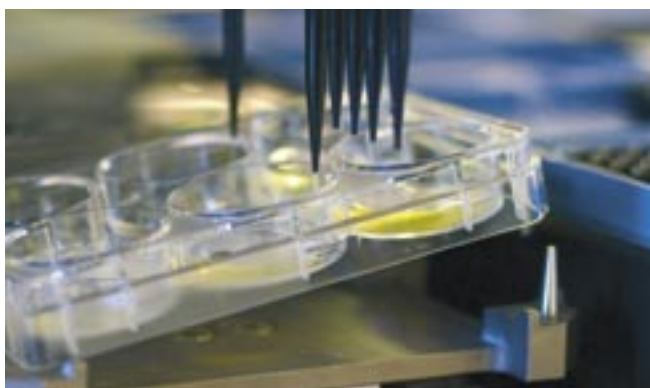
Figure 4: HAMILTON plate lifter mimics human manipulation of cell culture plates thus facilitating the complete removal of old medium.
