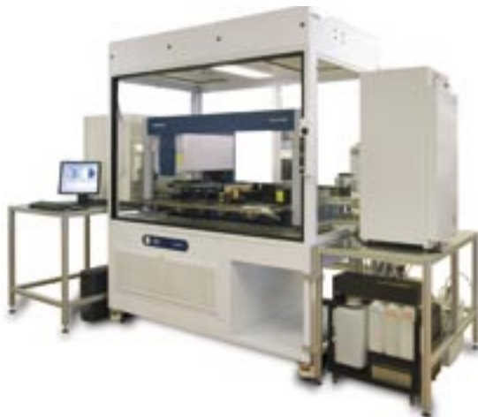
Figure 1: Cell host system. The core of the system is a MICROLAB ® STAR pipetting robot. Cell cultures and nutrient solutions as well as growth factors are kept in Kendro incubators at different temperatures (37°C incubator for cell cultures; 4°C incubator for media). The equipment is contained in a sterile housing with laminar air flow.
